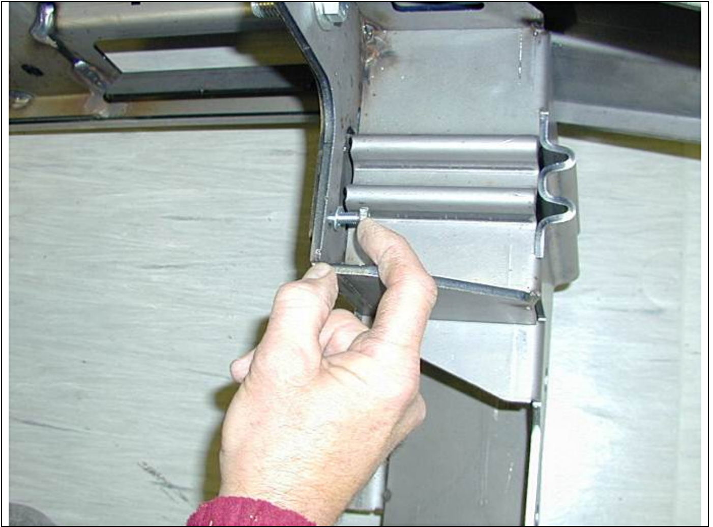
This photo shows the positioning of the 6mm bolt,nut etc to clamp the rear of the bull bar upright to the impact absorber.
